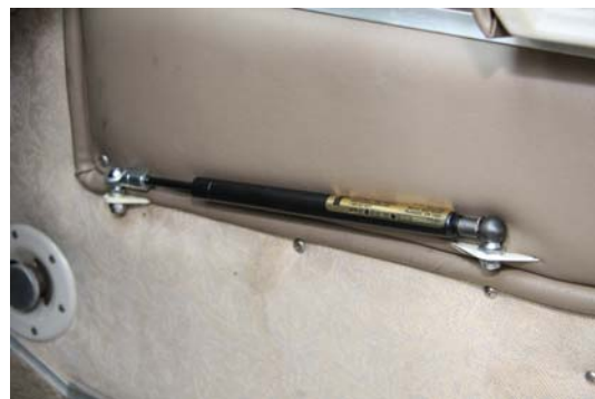
Picture 9. Closed Note door bracket mounted up slightly to avoid contact on the wind lace.
