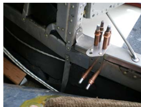
Picture 2. Airframe Bracket Clecoed in place.
