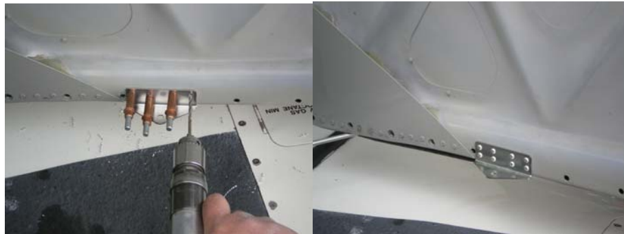
Picture 5. Drilling Door Bracket
