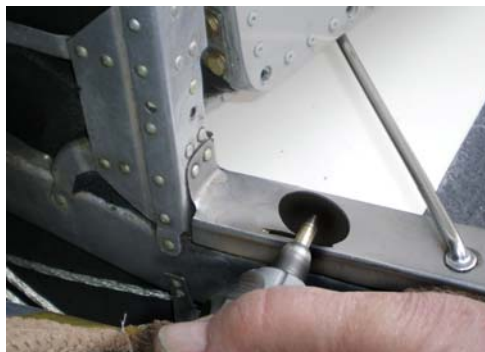
Picture 1. Cutting out sill area (Not Required on All Installations)
